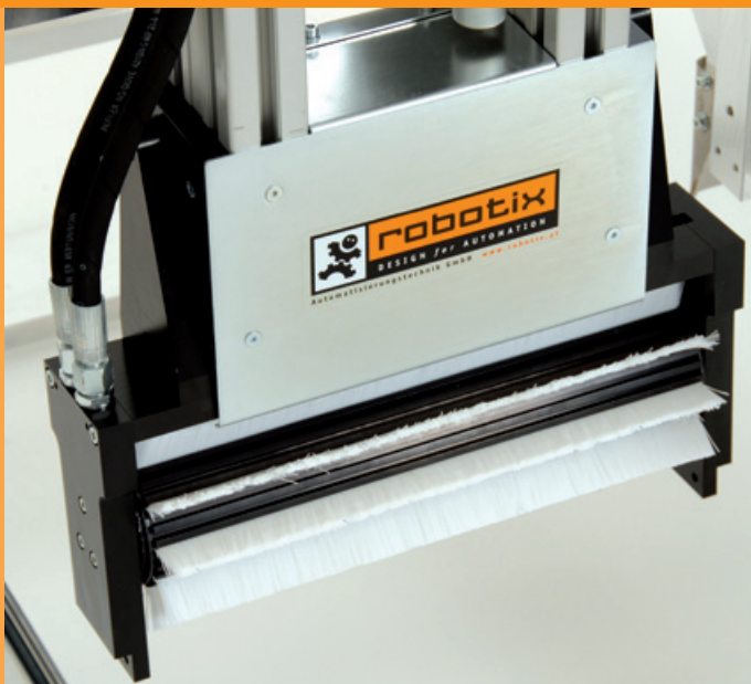
Hydraulic drive with pivot axis
